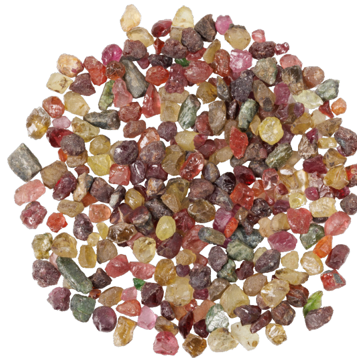
MGS 783 1 6. Wash pan concentrate of chrome-diopside, olivine and pyrope. Item belongs to the Mining Museum.
