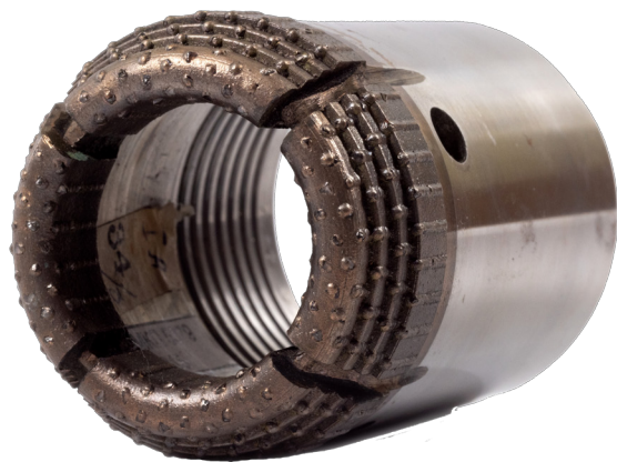
TI 215. Diamond bit SSK 59 1 for removable core receiver. Item belongs to the Mining Museum.
