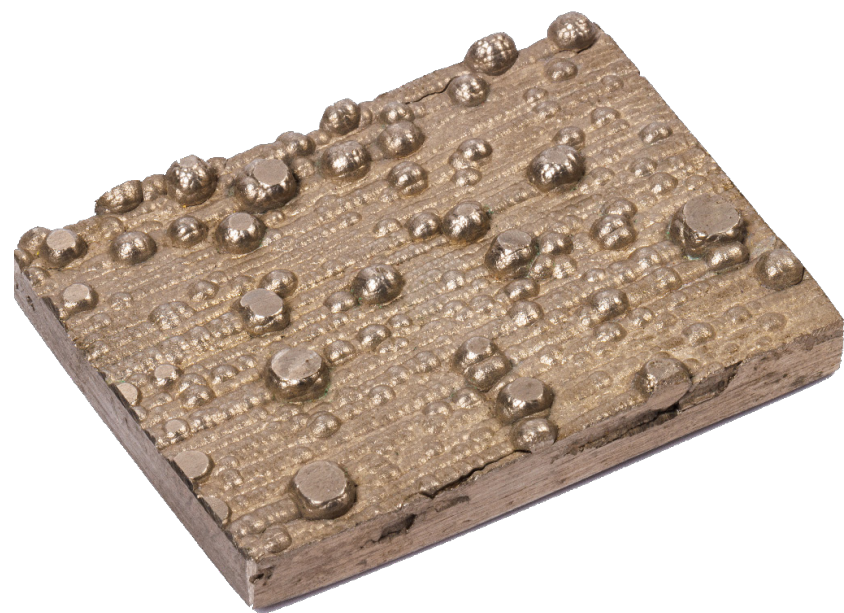
05 THS 7 7 Cathode nickel. Severonickel integrated plant. Item belongs to the Mining Museum.
