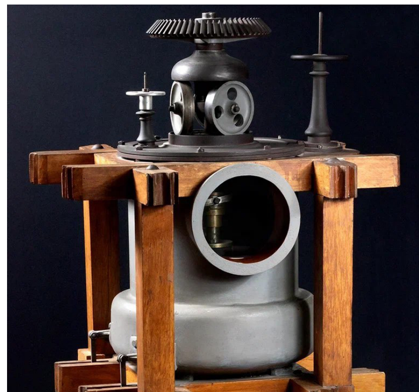
The model of a high pressure water turbine designed by Professor I.A. Time. Certified at the World's Fair in Vienna in 1873. F. Elery's machine shop. Saint Petersburg. Presented by Professor I.A. Time. Item belongs to the Mining Museum.
