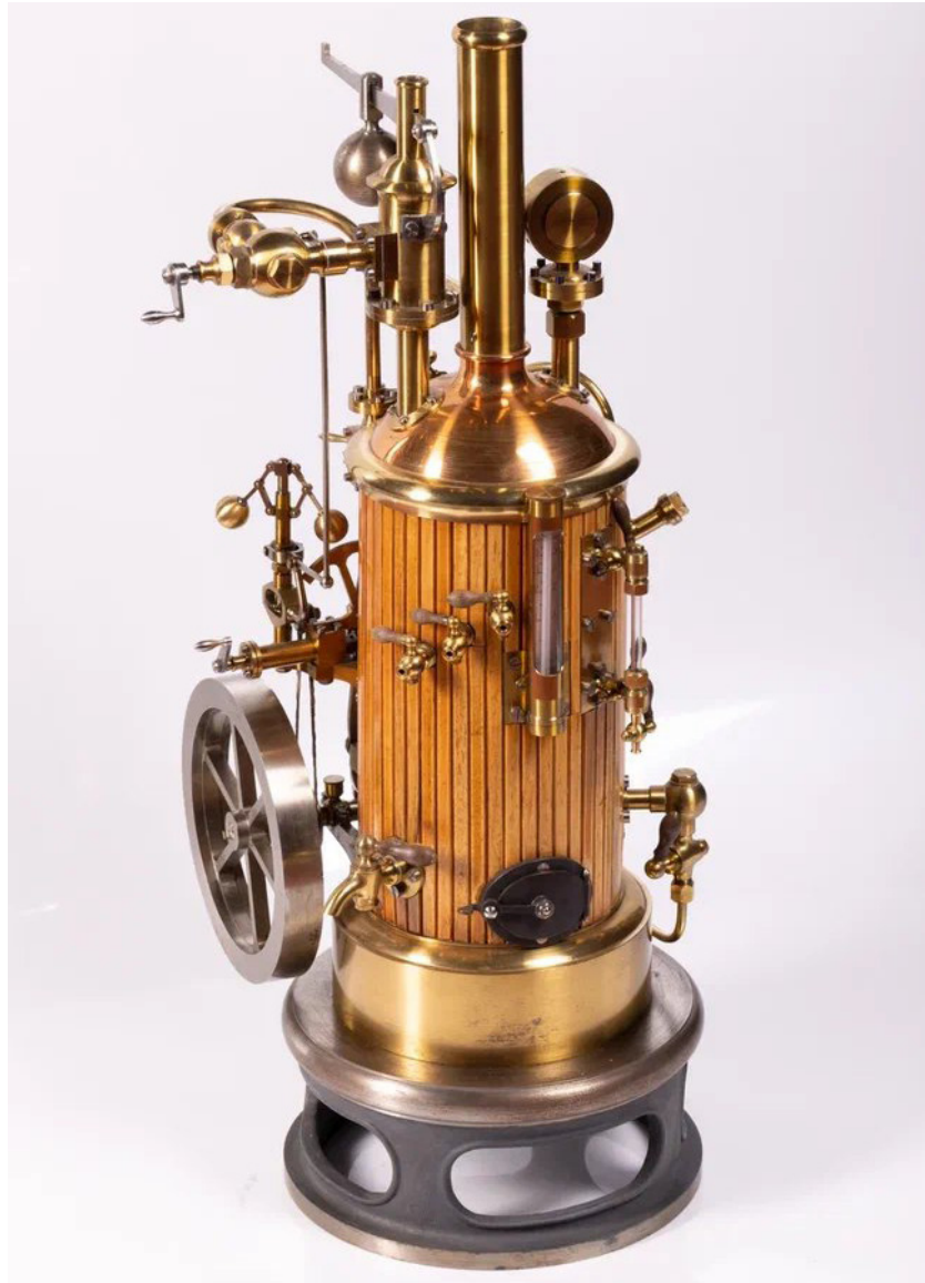
Model of a steam engine equipped with a vertical boiler. Peterman's machine shop. Saint Petersburg. Item belongs to the Mining Museum.
