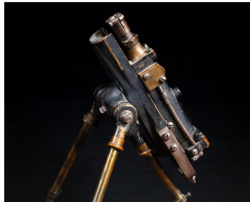
Model of a solenoid electric drill. Union Rock Drill, USA, 1870s. One of the first electric drills in the world. Scale 1:6. Presented by Engineer L. Nikolsky. Item belongs to the Mining Museum.
