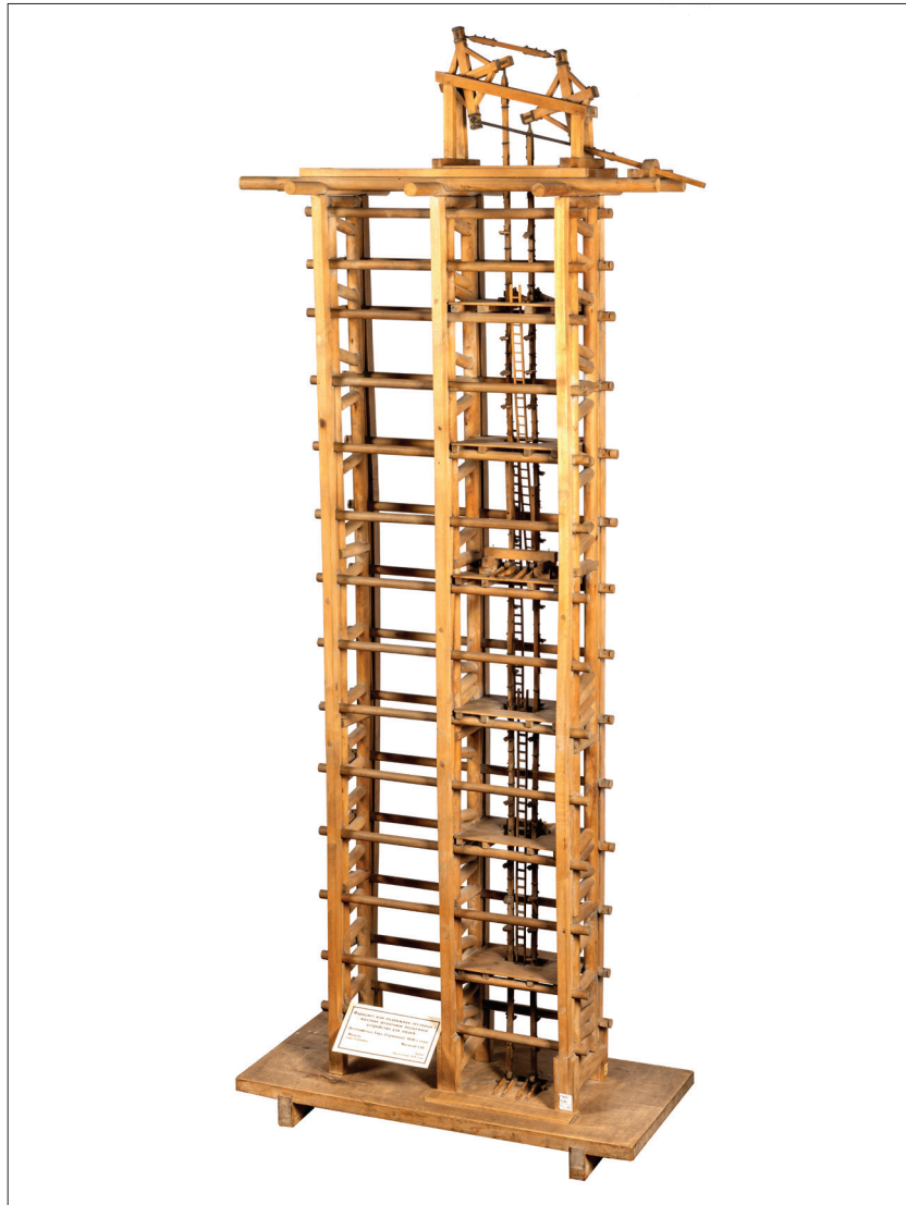
Fig. 1. Model of a man engine or mobile ladder is a mechanism of reciprocating ladders and stationary platforms installed in mines to assist the miners. 1830-s. Scale 1:16. Item belongs to the Mining Museum.
