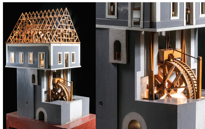
Fig. 2. Model of a lifting facility in mines equipped with a water wheel. Freiberg mines. Germany. 1830-s. Scale 1:20. Item belongs to the Mining Museum.
