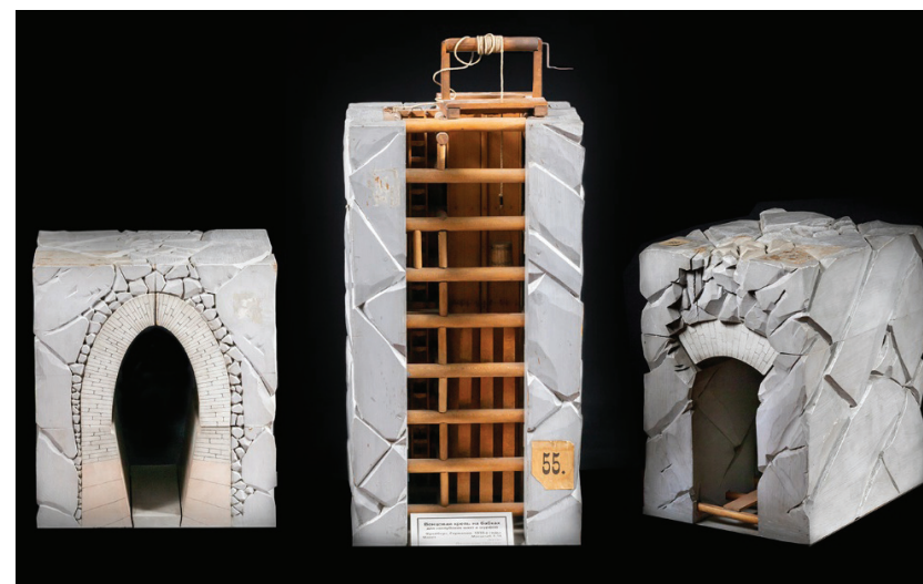
Fig. 4. Model of a curbing support for shallow mines and pits. Freiberg, Germany. 1830-s. Scale 1:16. Item belongs to the Mining Museum
