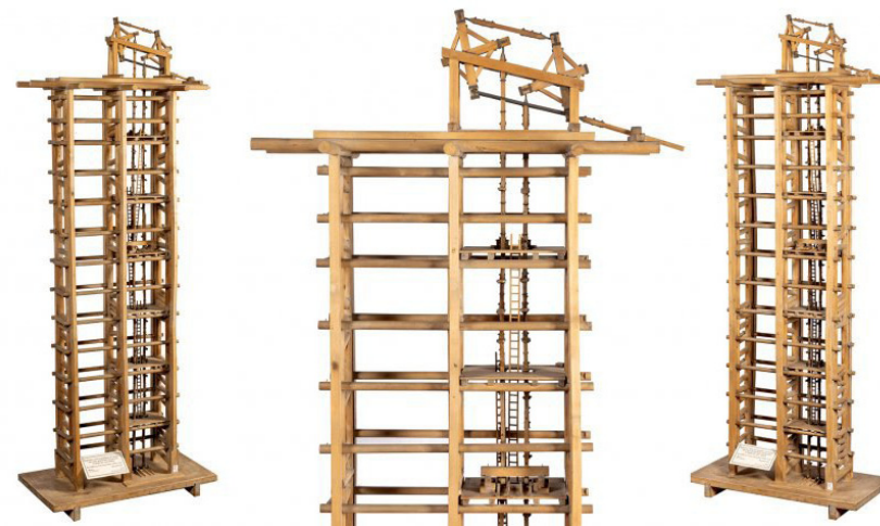
TI 80 Man engine or mobile ladder is a mechanism of reciprocating ladders and stationary platforms installed in mines to assist the miners. 1830s. Scale 1:16.
