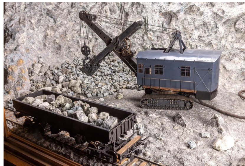
TI 191 Self-dumping car installed on two four-wheel trucks (Russia, mid-20 century) and a shovel excavator M-IV Э (TI 176 )in the apatite pit. (USSR. 1940. Scale 1:20). The model of first Soviet excavator.
