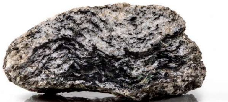
Amphibolite. Kola Superdeep Borehole. Depth: 11,260 m. From the collection of the Mining Museum
