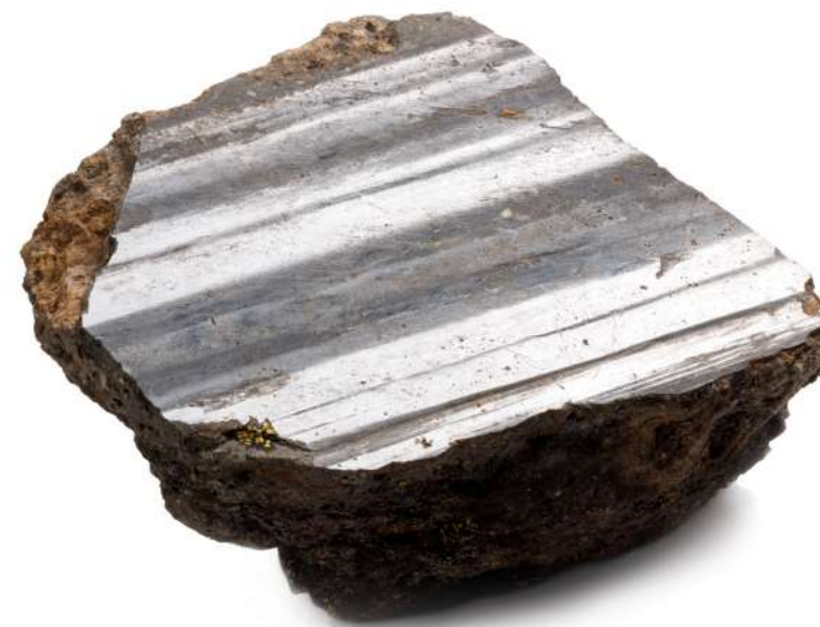
Slip surface in silicified sandstone. From the collection of the Mining Museum
