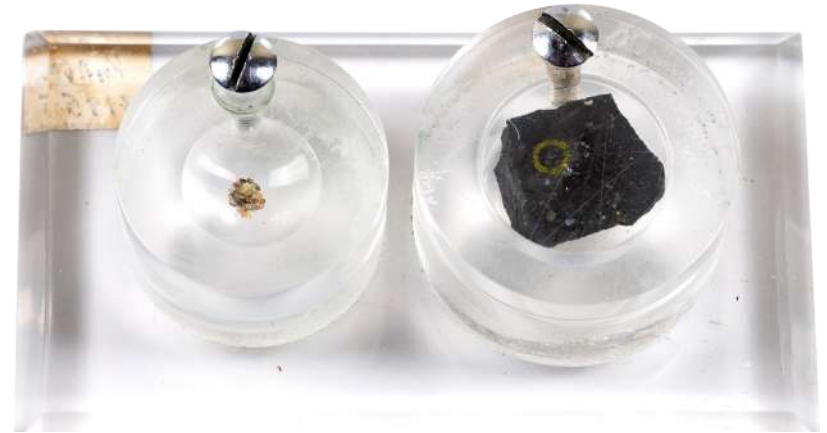
Impact diamonds in individual grains and an impact diamond grain in tagamite. Popigai Crater. From the collection of the Mining Museum
