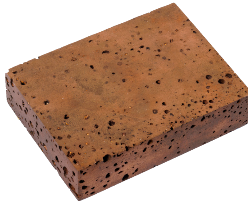
Anode copper. The Severnickel Integrated Plant. Item belongs to the Mining Museum.
