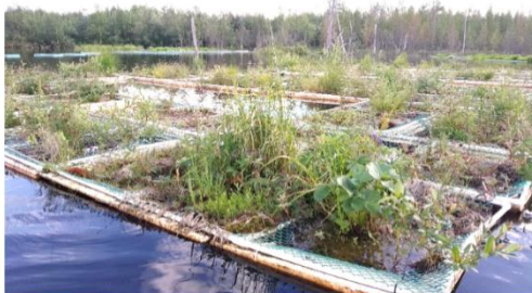
Fig.5. The state of phytocenoses created using different phytomodules: a – floating plant beds; b – bioplatform + grass turf; c – bioplatform + phytomats
