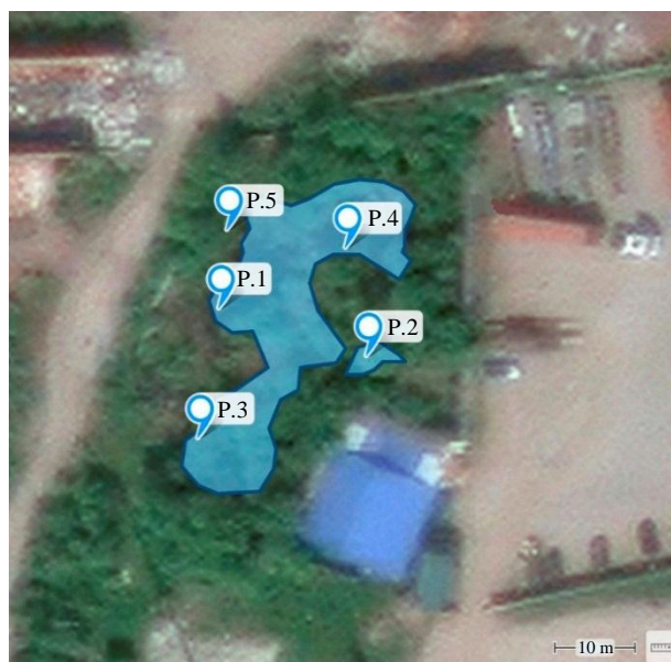
Fig.1. Map-scheme of soil sampling. Blue contour – localization of the spill; P.1- P.5 – Sampling sites
