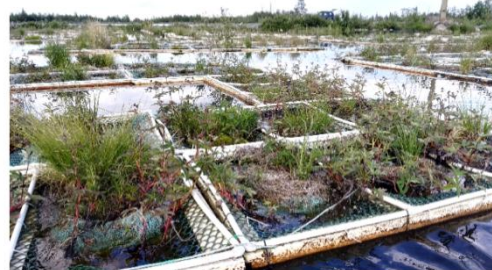
Fig.5. The state of phytocenoses created using different phytomodules: a – floating plant beds; b – bioplatform + grass turf; c – bioplatform + phytomats
