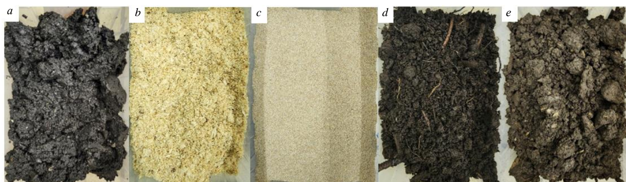
Fig.1. The appearance of the compostable mixture components: wastewater sludge (a), sawdust of pure wood (b), feed waste (c), peat (d), soil waste (e)
