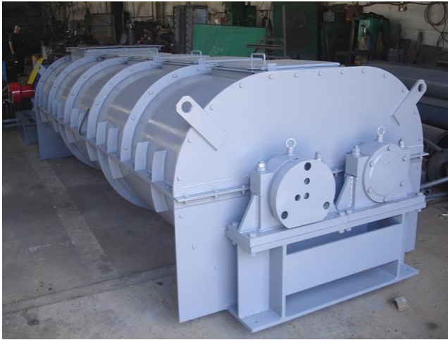
Fig.3. Twin-shaft paddle mixer SMK-126
