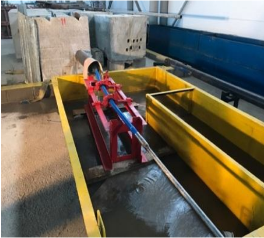
Fig.4. Bench testing of PDM operation
