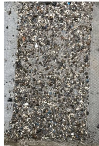
Fig.6. Photograph of the screen of the intake tank with the sludge from the bottomhole of the channel
