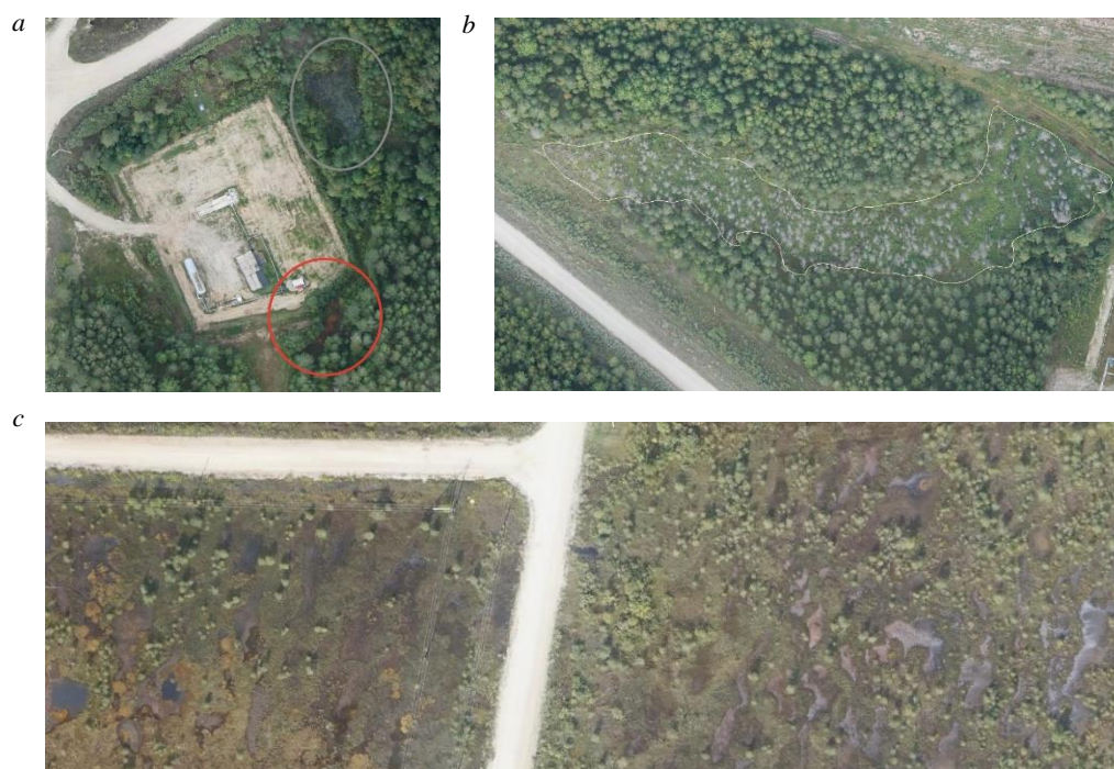
Fig.3. Fragments of the orthophotomap with areas showing signs of bitumization – black and dark red spots ( a ) and linearly elongated stripes of a drying up forest stand ( b ), halogenesis – a change in the reservoir colour to bluish-whitish in the right side of the picture ( c )
