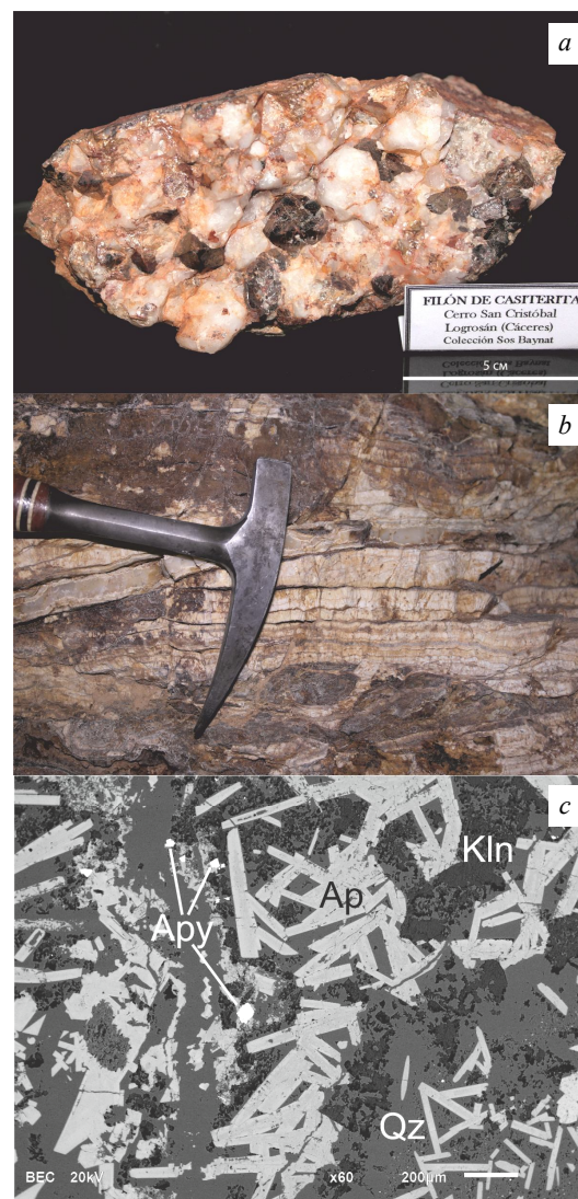
Fig.2. External appearance of the rocks under investigation: a – quartz-cassiterite druse from greisens, museum exhibit from Logrosán village; b – quartz-apatite vein, under exposure and through electronic microscope; c – image from back-scattered electrons
