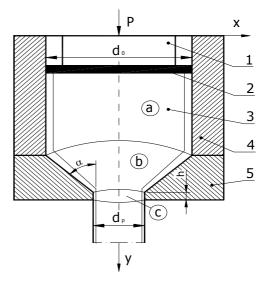
Fig.1. Schema direct extrusion of bimetal billet, 1- steam, 2- dummy block, 3- billet, 4- container, 5- die; a- deformation zone in container, b- deformation zone in die, c- sizing zone;  $d_0-$  initial diameter of billet,  $d_p-$  final diameter,  $\alpha-$  half conical die angle, b- high of sizing zone
