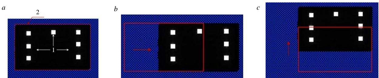
Fig.5. Verification of the reference position of point light sources by the machine vision system: a – reference position of the CMP; b – horizontal region of interest definition; c – vertical region of interest definition 1 – reference position of the fiducial markers; 2 – rectangular region of interest
