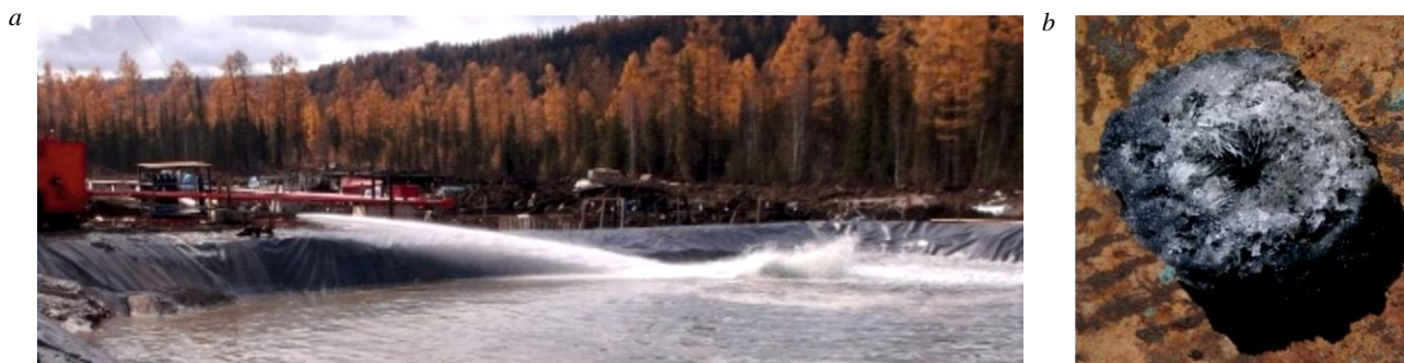
Fig.1. Kovykta area, Angara-Lena artesian basin: a – controlled free-flowing of a deep well, “Lithium” site; b – salt plug inside drill pipes – salts crystallize when the system’s PVT conditions are disrupted (photos provided by A.G.Vakhromeev)
