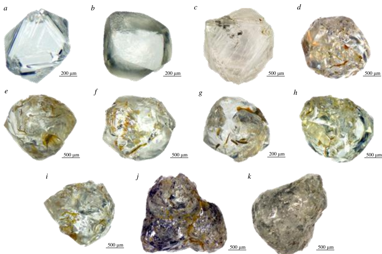
Fig.2. Typical diamond crystals of the studied collection a-c – diamonds of the variety I according to Yu.L.Orlov: a, c – a colorless octahedron with polycentrically growing edges, b – curved dodecahedron; d-i – curved dodecahedron with deep scars on the surface filled with ironification products; j, k – diamonds of V-VII varieties with numerous dark-colored inclusions
