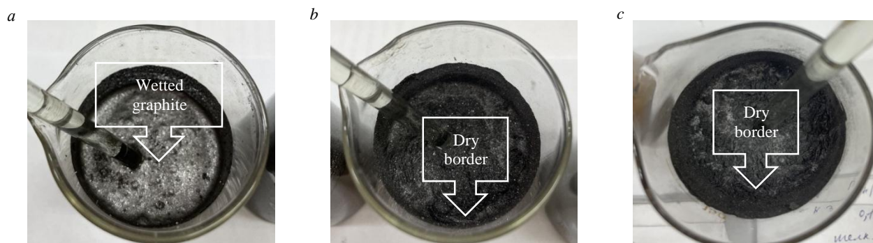
Fig.3. Photographs of interaction of ESS dust ground in a ball mill ( a ), from coarse ( b ) and fine ( c ) classification products in the GC-0.36 complex with water
