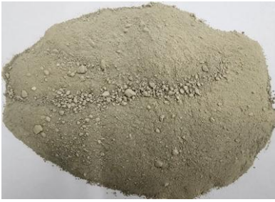
Fig.7. Bulk material based on landfill leachate and blast furnace slag
