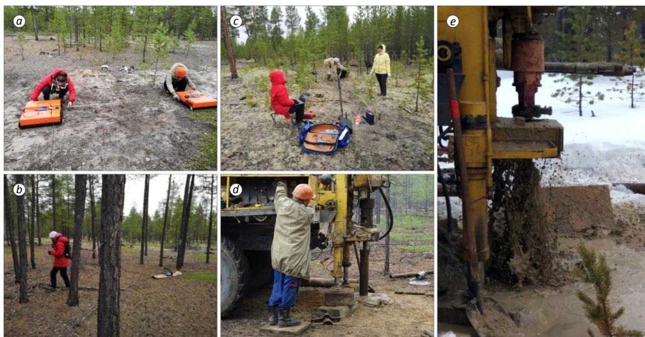
Fig.2. Progress of CDP ( a ), GPR ( b ), electrical exploration ( c ), drilling ( d ) and a fountain of water gushing from a drilled well ( e )
