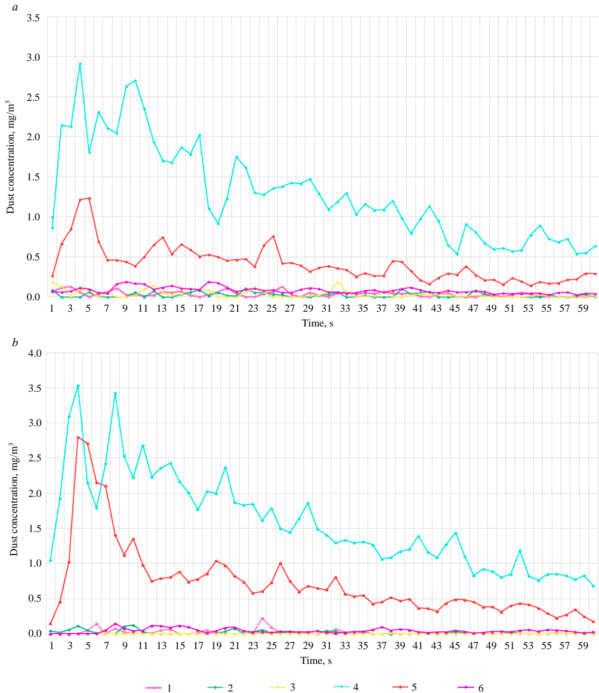
Fig.5. Graphs of the dependence of the total concentration of dust particles on time during instantaneous measurement (a) and 20 min (b) after irrigation of sulfur with the tested compounds 1-6
