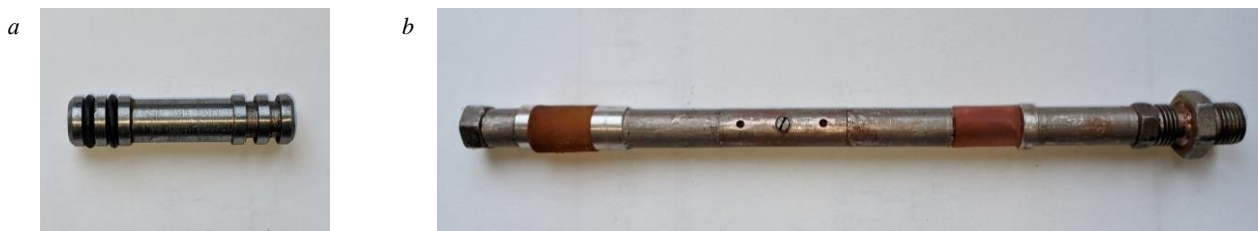
Fig.2. Sealing device for isolating an inclined borehole (a) and a double packer tool (b)
