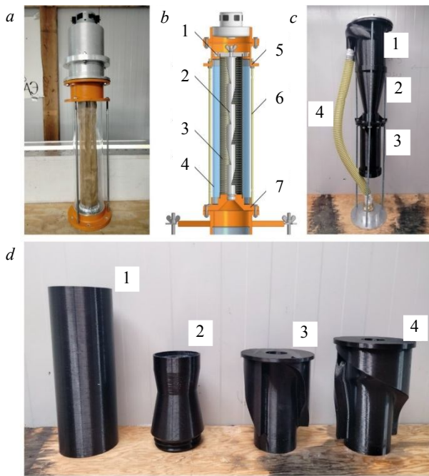
Fig.6. Designs of cuttings collection filters: a – general view of the experimental stand upper part before testing the mesh cuttings collection filter; b – mesh cuttings collection filter (1 – mesh filter flange; 2 – sludge lifting tube; 3 – mesh filter; 4 – transparent plexiglass pipe; 5 – top flange; 6 – studs; 7 – lower flange); c – cyclone filter with one inlet pipe (1 – cylindrical part of the cyclone with tangential supply; 2 – conical part of the cyclone; 3 – sludge collection tank; 4 – sludge lifting hose); d – cyclone filter with two and three inlets (1 – sludge collection tank; 2 – conical part of the cyclone; 3 – upper part of the cyclone with two inlets; 4 – top part of a cyclone with three inlets)
