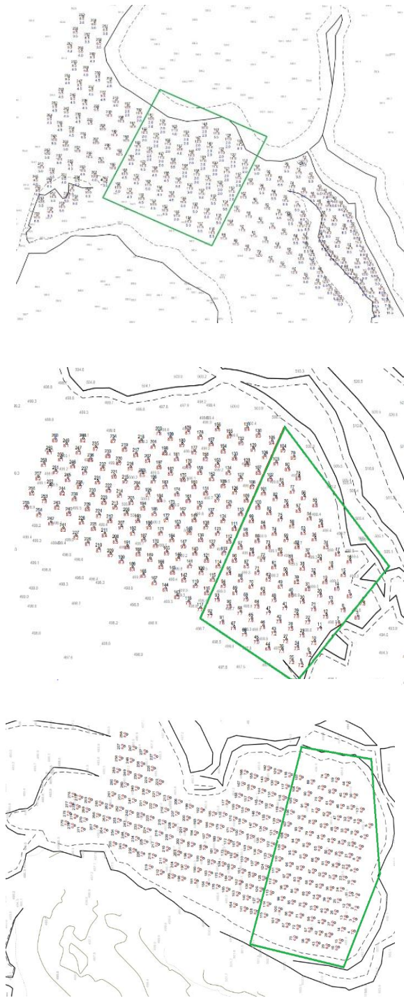
Fig.4. Location plans of drilling and blasting wells on the experimental blocks (green contour are areas where explosive charging was done according to the specific energy consumption of drilling)
