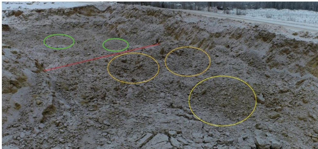
Fig.5. Results of drilling and blasting on the experimental block (yellow color indicates funnels with standard parameters, green – with experimental ones)
