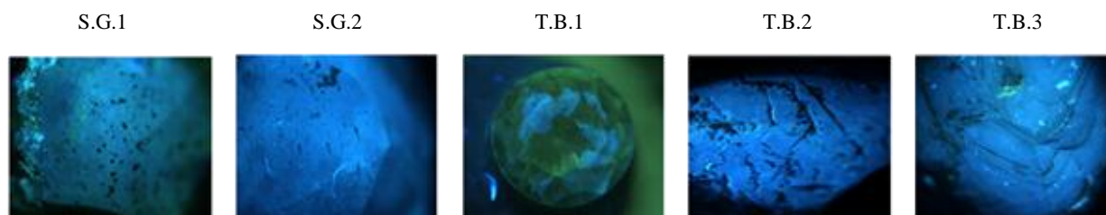
Fig.2. Luminescence images of diamonds under Diamond View (UV < 230 nm)
