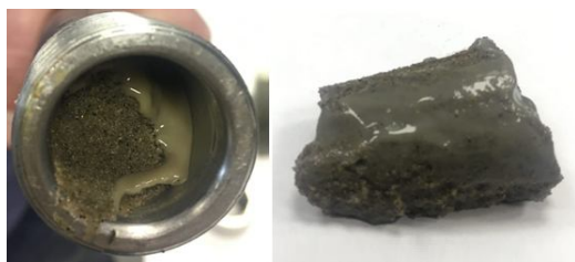
Fig.4. A jellylike layer of technical grade LS removed from disassembled tube
