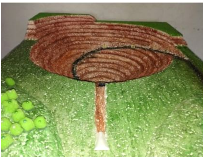
Fig. 5. Model of the quarry with ventilation passage
