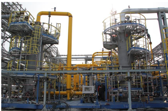
Fig.2. Experimental installation for low-temperature separation with plate heat-exchangers
