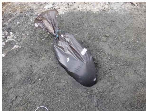
Fig.5. Shell is installed in a dry well and filled with water
