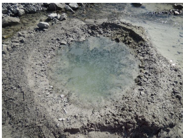
Fig.4. A 10 m well filled with drill fines and water. Well top is absent
