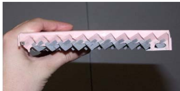
Fig.4. Hybrid structure made of topologically interlocked metallic cubes with flexible polymer base [9]
