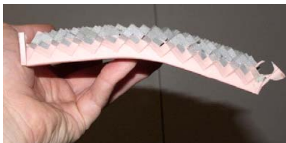
Fig.4. Hybrid structure made of topologically interlocked metallic cubes with flexible polymer base [9]
