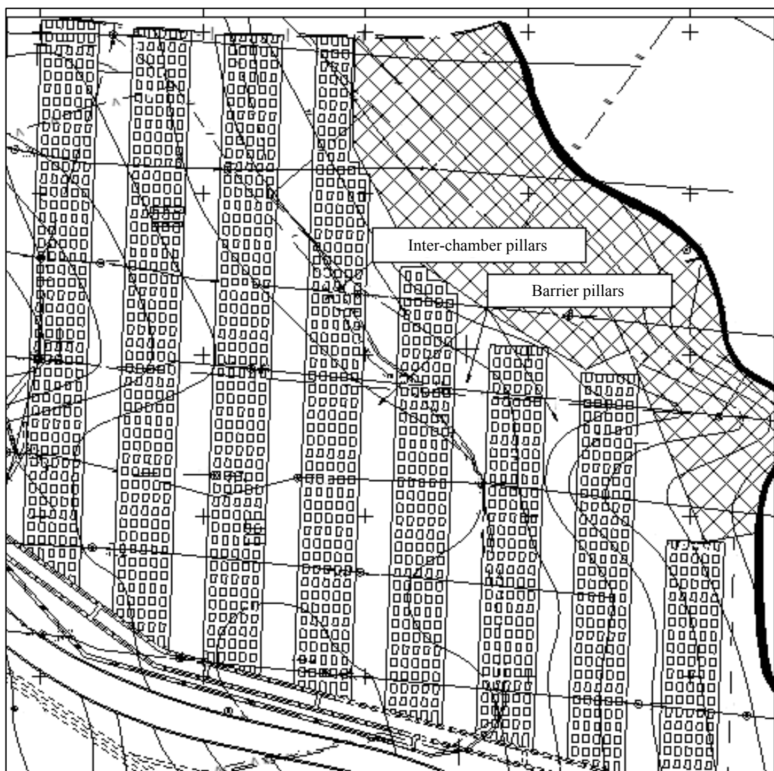
Fig.3. Layout of Nui Beo mine section developed with short longwall faces
