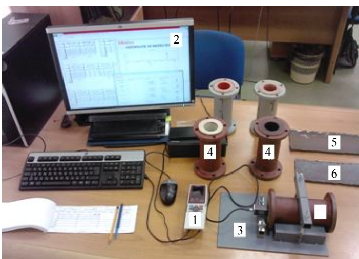
Fig. 2. General view of measuring unit 1 – profilometer; 2 – PC; 3 – logement; 4 – test samples with polyurethane lining; 5 – a piece of steel pipe (new pipe); 6 – a piece of steel pipe with run in roughness (used pipe)
