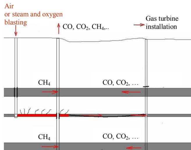
Fig. 4. Periodic intensification of degassing by sending combustion products through the seam
