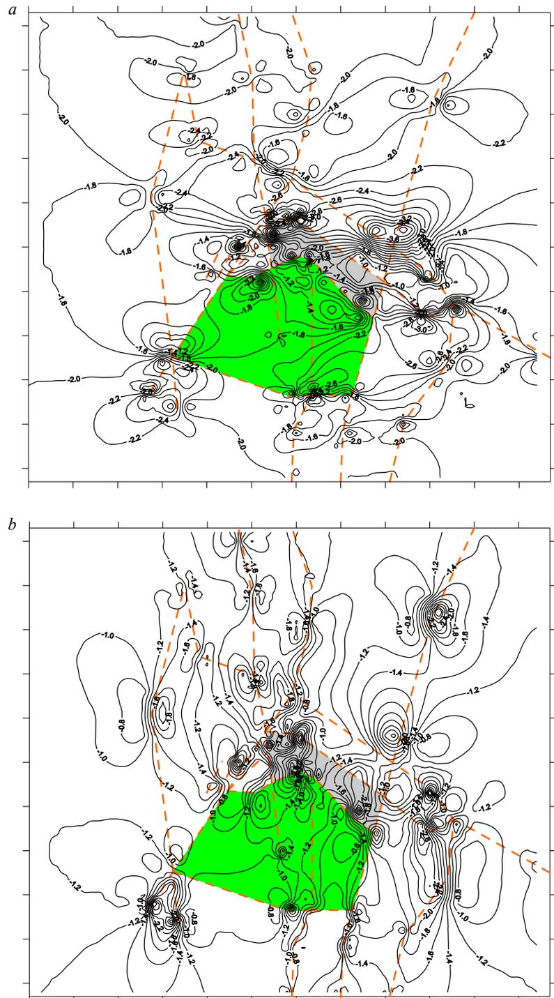
Fig.1. Prognostic map of tensed state  $\sigma_x$  (a) and  $\sigma_z$  (b) the block massif of rock types of the Talda zone, Kuzbass
