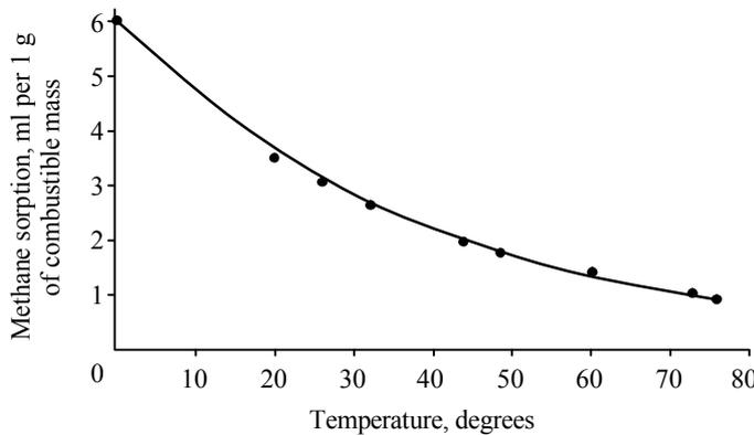
Fig.3. The dependence of coal sorption capacity on temperature
