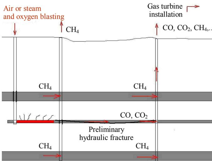
Fig.2. Degassing via in situ gasification of one of the lower weak coal beds in the suite
