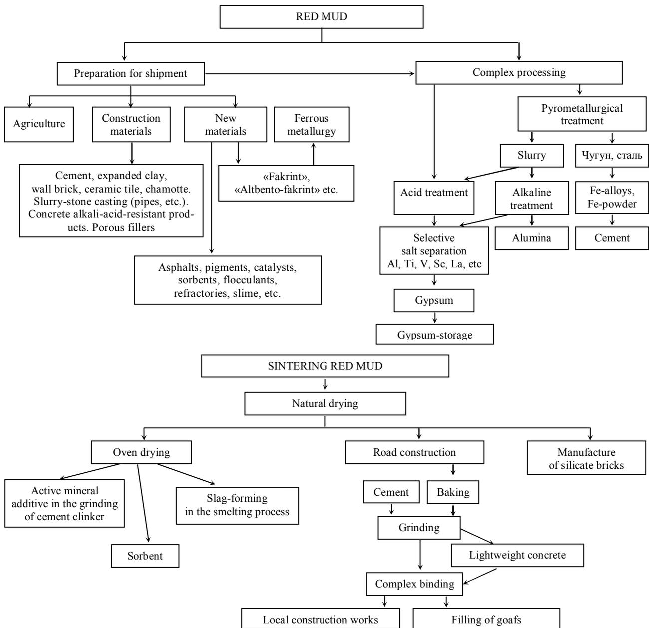
Fig.2. The most promising and proven ways of processing red mud
