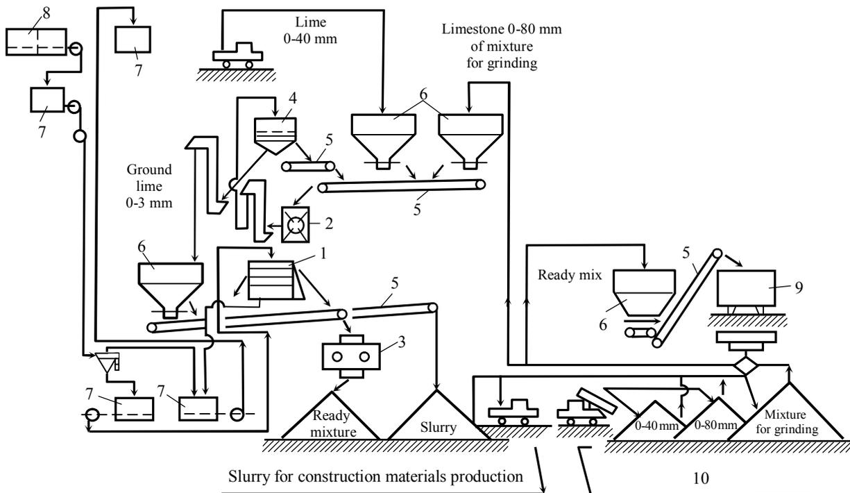
Fig.3. Equipment-technological scheme of the main industrial plant for production of transportable red mud product with capacity more than 20 thousand t/year
