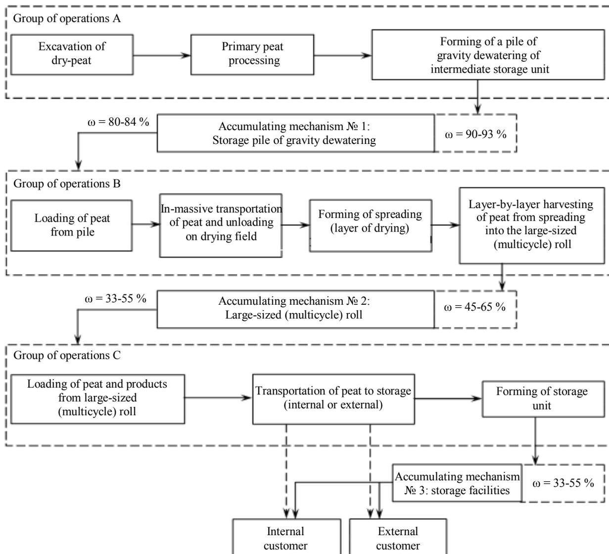
Fig.8. Structure of complex of technological operations for peat excavation with the stage dewatering in the spreading and intermediate storage units
