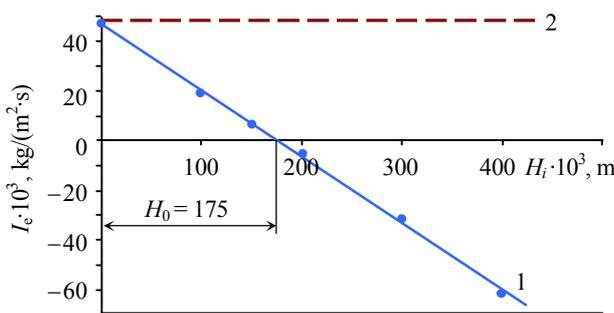
Fig. 3. Pattern of evaporation rate, thickness of pile of terrestrial peat  $R_r = 22-25\%$  (1) and maximum value  $i_e = \alpha_R B$  (2)
