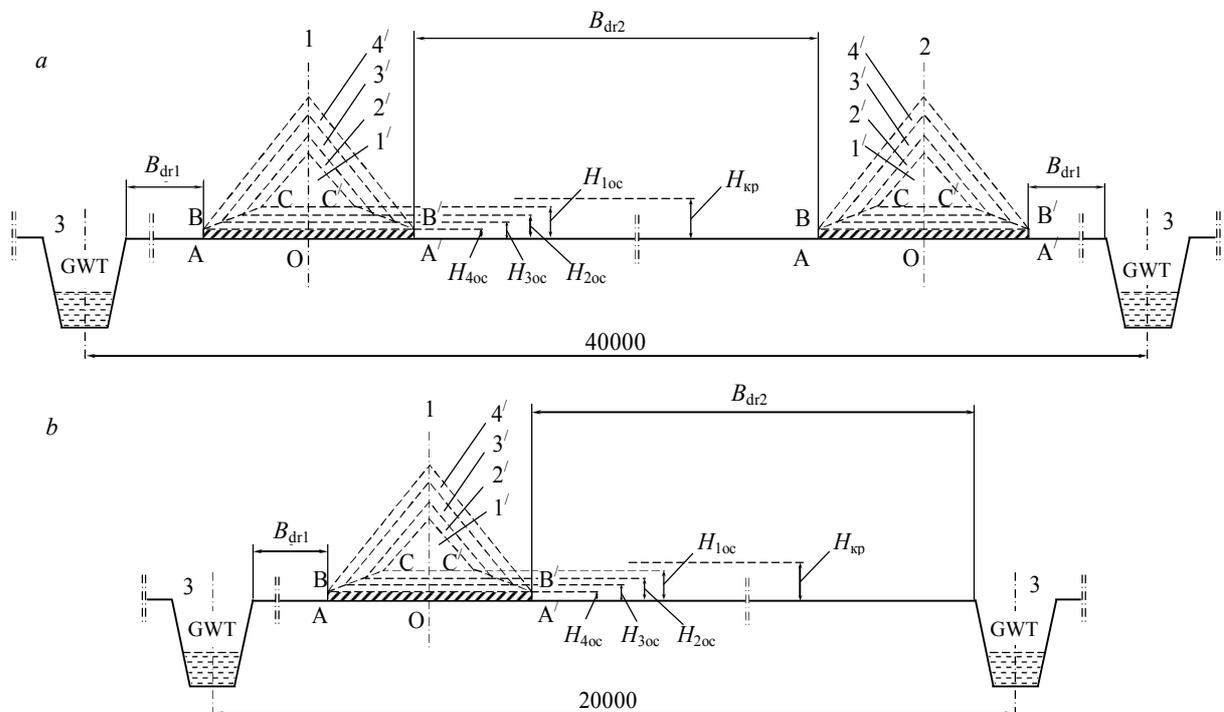
Fig.7. Scheme of location of large-sized rolls (4 harvestings) for lowdown (a) and terrestrial (b) peat deposit
