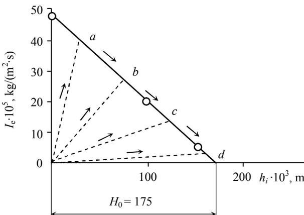
Fig. 4. Scheme of smoothing the maximum (a, b, c, d) for patterns of evaporation rate and height of pile (layer) of peat materials (processing of data at fig.3)
