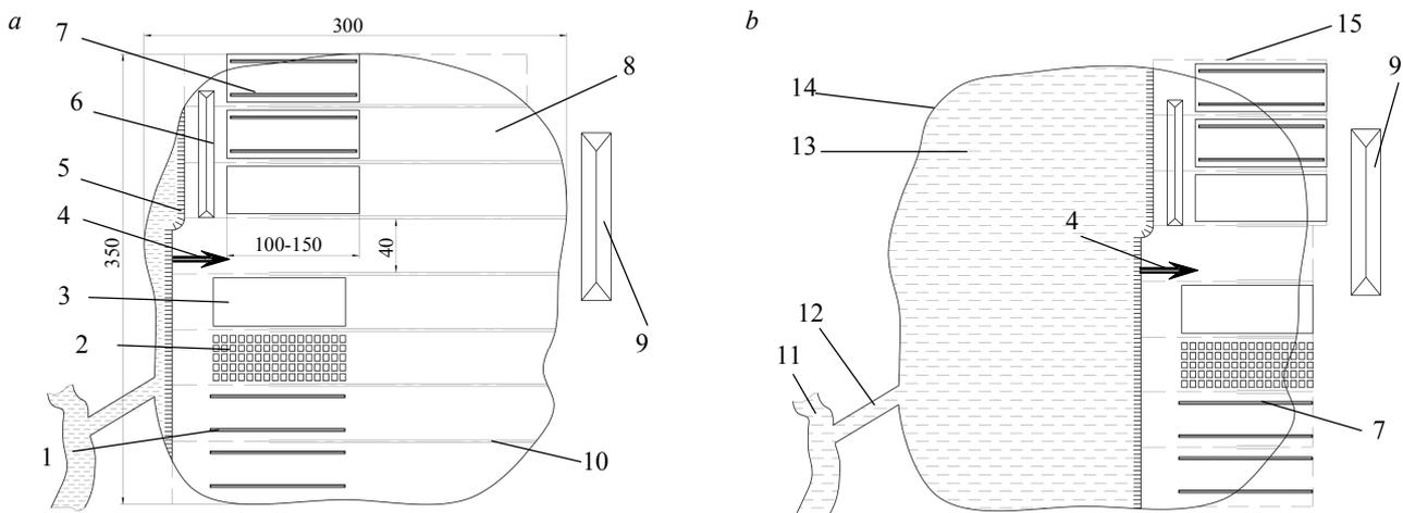
Fig.9. A scheme of technological area of peat excavation with stage dewatering in the spreading and intermediate storage units (during initial period of exploitation (a) and final (b) period of pile exploitation)
