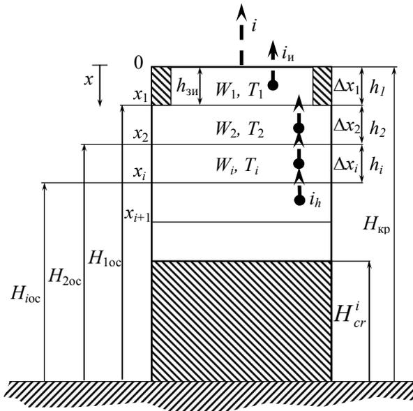
Fig. 2. Scheme of layers location in the pile of peat of critical thickness during drying ( $|i| = |i_{gl}| + |i_{ul}| + |i_{hl}|$ )
