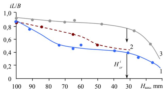
Fig.5. Relative heat costs for moisture evaporation  $iL/B$  for peat drying in thick layers
