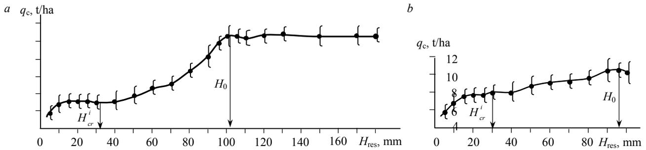
Fig.6. Cyclic harvesting of peat and thickness of aeration layer (without turning): a – data of 2013; b – data of 1981
