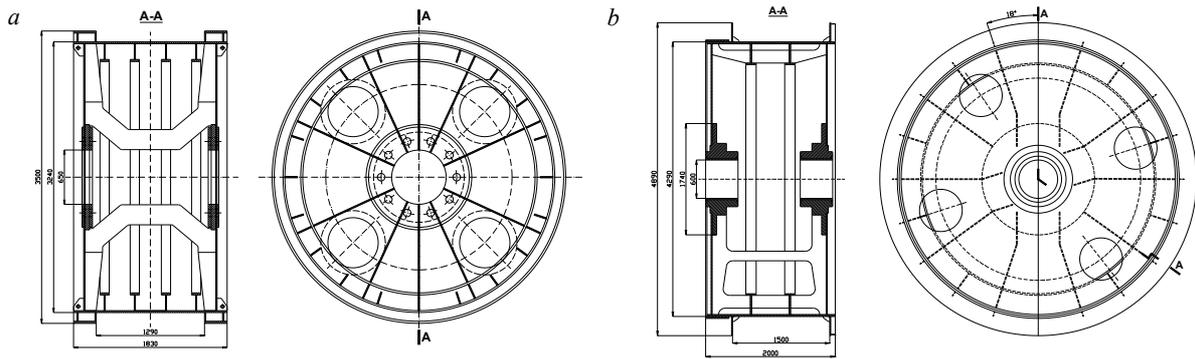
Fig. 1. Drums drafts: *a* – frictional type; *b* – rolling type
