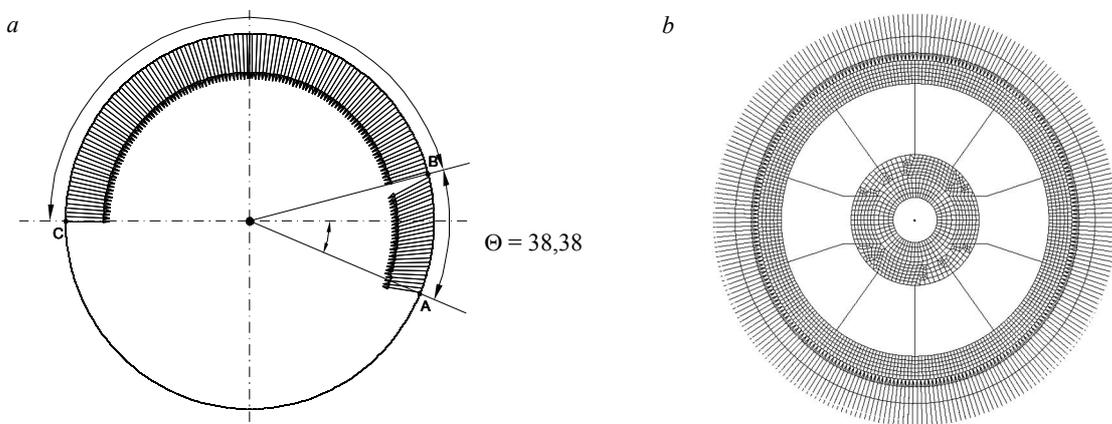
Fig. 2. Loads scheme: *a* – frictional type; *b* – rolling type
