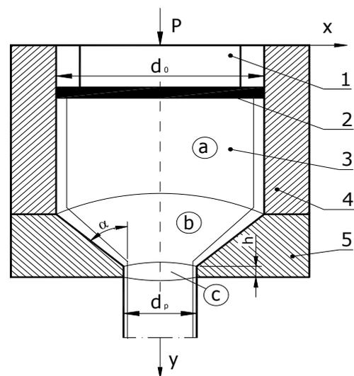
Fig. 1. Schema direct extrusion of bimetals billet, 1 – steam, 2 – dummy block, 3 – billet, 4 – container, 5 – die; a – deformation zone in container, b – deformation zone in die, c – sizing zone;  $d_0$  – initial diameter of billet,  $d_p$  – final diameter,  $\alpha$  – half conical die angle,  $h$  – high of sizing zone
