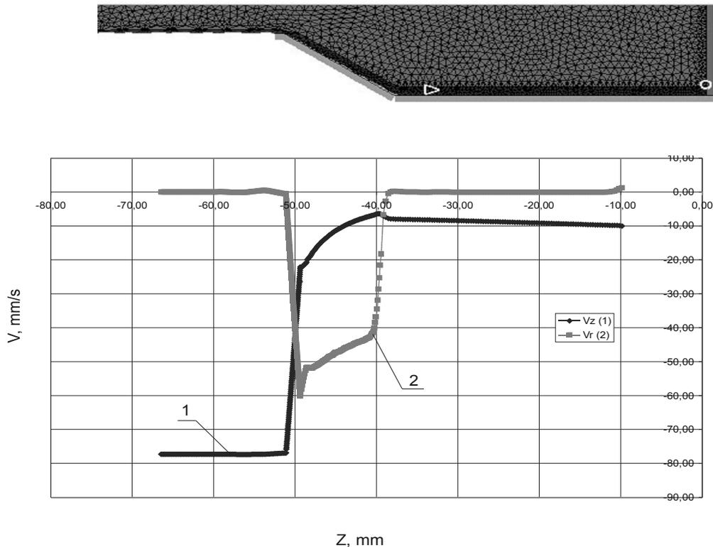
Fig.2. Changing the values of longitudinal  $V_z$  velocity component radial  $V_r$  during the bimetallic extrusion of Al/Cu rod in the contact zone between die and billet (FORGE2 model)
