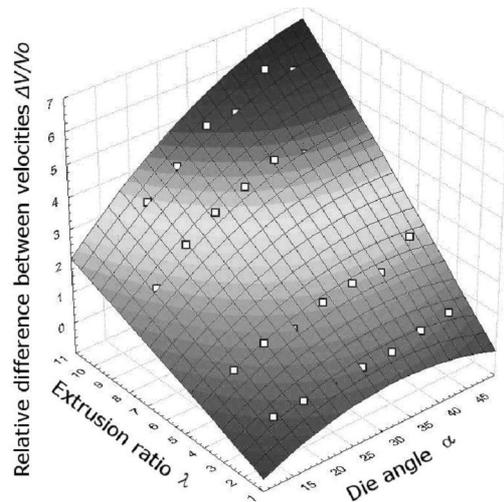
Fig.5. Relationship between the extrusion ratio  $\lambda$  and die angle  $\alpha$  and maximal differences in velocities in axis, and velocities in boundary layers
