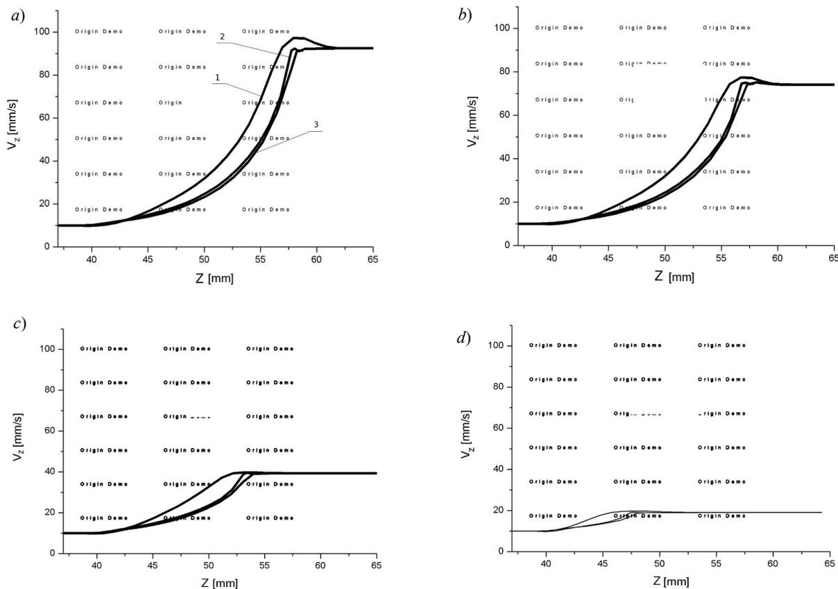
Fig.3. Velocity of bimetal flow in billet axis (1), in the boundary of layer contact (2) and in the surface of contact between billet and layer (3), with half die angle  $\alpha = 15^\circ$ , with extrusion ratios: a)  $\lambda = 10$ , b)  $\lambda = 8$ , c)  $\lambda = 4$ , d)  $\lambda = 2$
