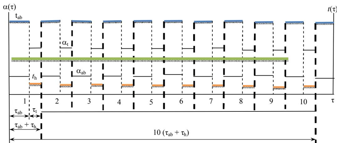
Fig.1. Temperature (solid lines) and heat exchange coefficient (dashes) changes at the incoming part of working during winter period
