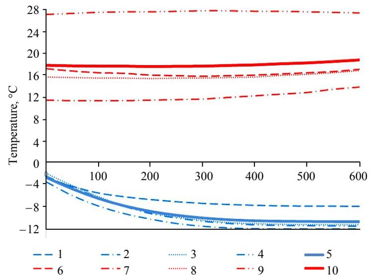
Fig.9. Dynamics of air flow temperature in control cross-section points and its averaged values along the working cross-section (blue – temperature of preheated air at tunnel entrance, red – at cross-section, where the preheated air is injected)
