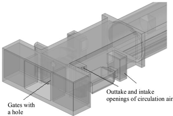
Fig.5. External view of Baikal tunnel portal with ventilation gates and air preheating and injection system
