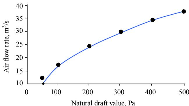
Fig.7. Relationship of tunnel incoming air rate from natural draft value (solid line – mathematical modelling results; dots – calculation results from experimental identification of local resistance coefficient)
