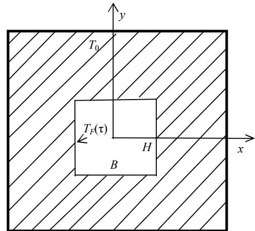
Fig.2. Calculation scheme for describing heat exchange process between air flow and roof support surface
