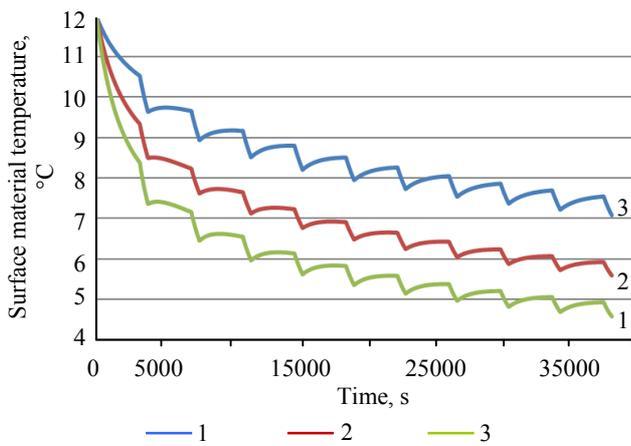
Fig.3. Concrete support surface temperature during periods of 3200 and 600 with corresponding heat transfer coefficients  $\alpha_{ab}$  and  $\alpha_t$
