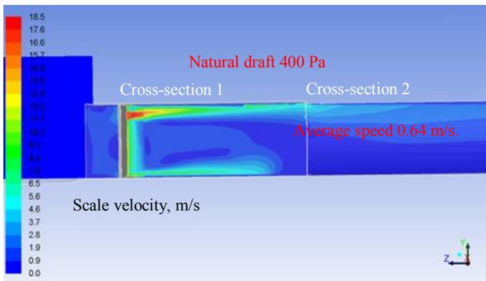
Fig.6. Distribution of air flow rate in cross-section near ventilation gates of western portal and with natural draft value of 400 Pa
