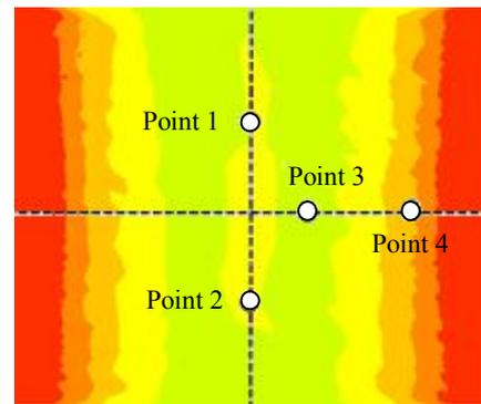
Fig.8. Placement of control points in working cross-section with injection if preheated air and distribution of temperatures
