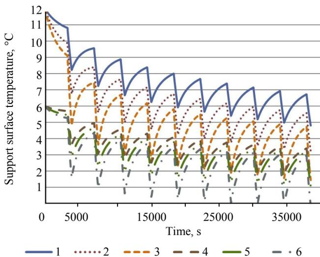
Fig.4. Support surface temperature in relation to time and heat transfer coefficient value
